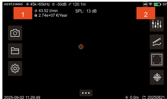
3.1.2-Gas Leakage Detection Interface
