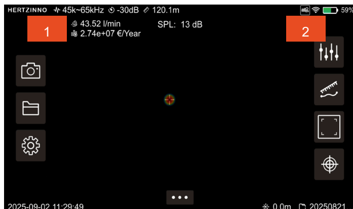
3.1.2-Gas Leakage Detection Interface
